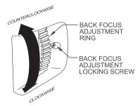
Figure 7. Back Focus Adjustment
